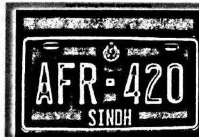
Fig. 2. Output binary image for Mean adaptive thresholding
